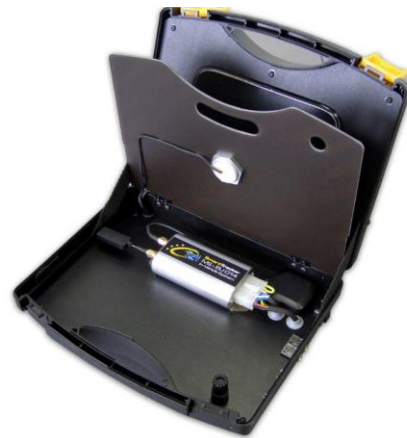
Fig. 5. The EuroGPS SmartTracker IVS-EU014 eCall System [13].
