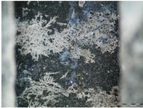
Fig. 7. Dendrite and blue colored residues formed in 1 mM NaCl solution during WD test in case of Sn sample.
