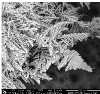
Fig. 1. Scanning electron microscope (SEM) image of dendrites.
