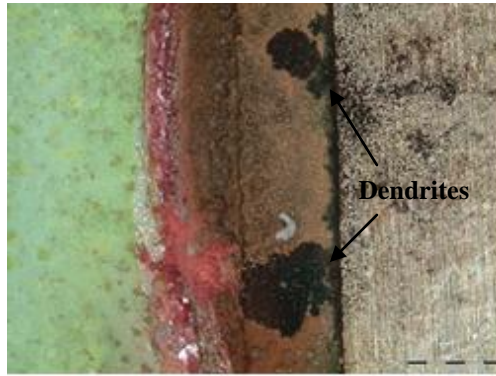
Fig. 10. Dendrites formed in 500mM NaCl TEL during WD test in case of immersion silver.
