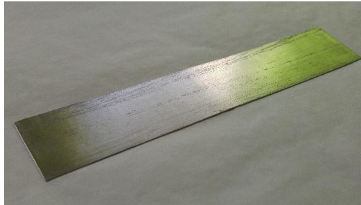
Fig. 4. Sn-Sn solder alloy plate after rolling.
