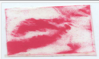
Figure 2a: A single sheet Fuji Pre-scale Film was used to record the pressure inside the non-union area and beneath the plate. Fuji Pre-scale Film: Mitsui & Co, Los Angeles, USA, PPF.
