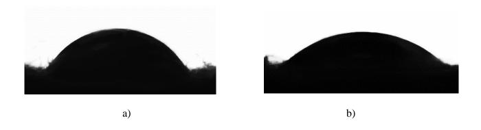
Fig. 4 Diiodomethane contact angles on the surface of raw cotton (a) and linen (b) fabrics
