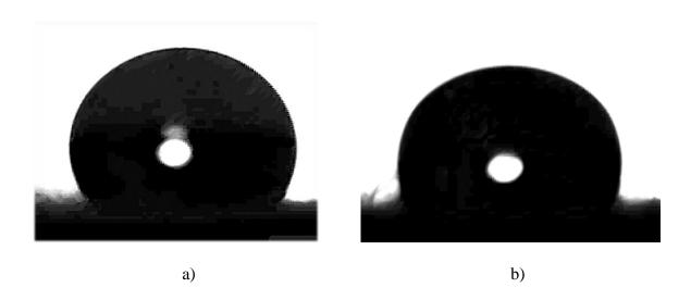
Fig. 3 Water contact angles on the surface of raw cotton (a) and linen (b) fabrics
