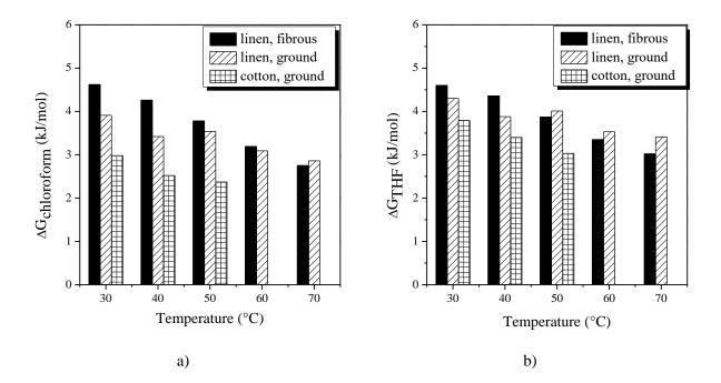
Fig. 5  $\Delta G_A{}^{ab}$  of chloroform (a) and THF (b) adsorption at different temperatures for fibrous and ground linen and for ground cotton
