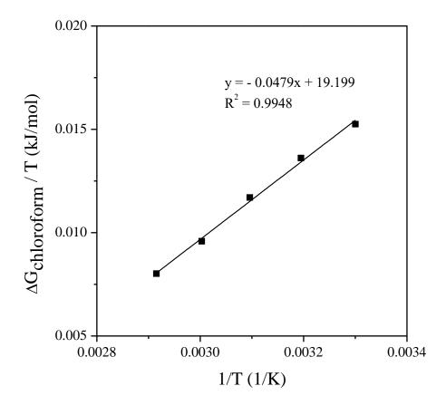
Fig. 7 Determination of specific enthalpy of adsorption of chloroform on linen fibre
