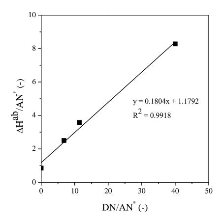
Fig. 8 Determination of acid-base constants of linen fibre
