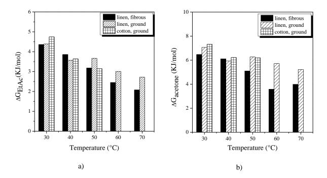
Fig. 6  $\Delta G_A{}^{ab}$  of adsorption of amphoteric probes (a: ethyl acetate, b: acetone) at different temperatures for fibrous and ground linen and for ground cotton
