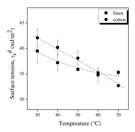
Fig. 2 Effect of temperature on the dispersion component of surface tension  $(\gamma_s^d)$  of ground cotton and linen samples
