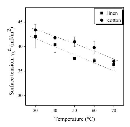
Fig. 1 Effect of temperature on the dispersion component of surface tension  $(\gamma_s^d)$  of fibrous cotton and linen samples
