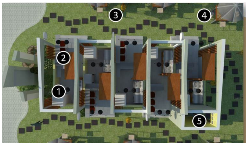
Fig. 9. The Plan of the Hawker Centre Design [Legend: 1. Kitchen, 2. Indoor Eating Area, 3. Outdoor Eating Area, 4. Playground, 5. Toilet] (Source: Author)
