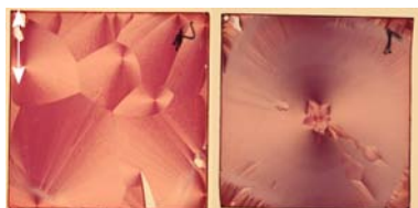
Figure 7.18: Comparison between several randomly nucleated spherulites, or a single centered one. Samples are 25 by 25 mm 2 in size.
