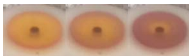
Figure 7.4: The drying process during regular spin coating. The three subsequent still images span 1 s.
