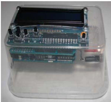
Figure A.4: Photo of the custom-made voltage source inside its case made from a repurposed box of candy.
