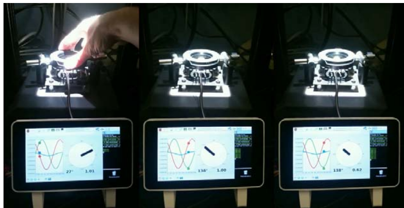
Figure 8.13: Still images of a video demonstrating the real-time determination of irradiance and the angle of polarization of incident light. The three colored points represent the measured J_{sc} . Only a single angle exists where all three points coincide with the calibration curves. The black clock hand represents the light intensity and angle of polarization as determined by least squares fitting. Between the first and second frame, the angle of polarization was changed. Between the second and the third, the incident irradiation was decreased.
