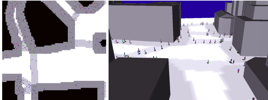
Figure 2.3: On the left, the 2D color map encodes the ground (white), buildings (black), sidewalks (dark gray) and crossings (light gray). On the right, an example of a simulation in a urban virtual environment. ( Loscos et al., 2003 [56] )
