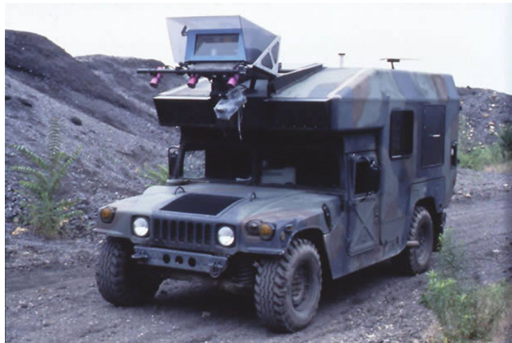
Figure 2.23: The Navigational Laboratory II (NAVLAB II) was the robot used for testing the capabilities of the proposed algorithm. It successfully found a path between the initial position and a goal position set in an unknown area of 500 x 500 meters. (Stentz et al., 1995 [81])
