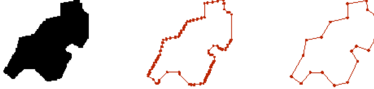
Figure 4.6: A polygon on the Binary Partition (Left); A high density pre-simplified polygon (Center); The final simplified polygon (Right).
