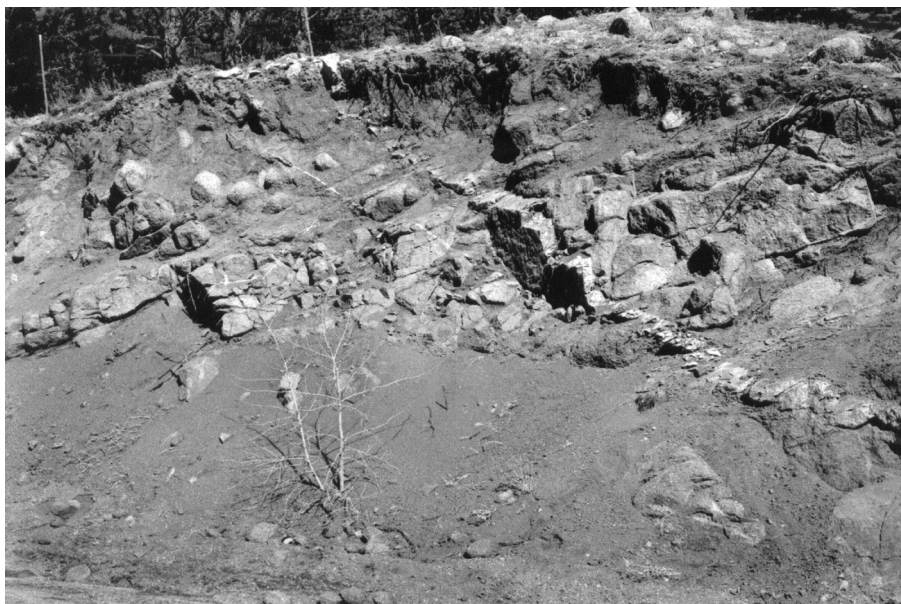
Figure 7c. Small corestones exposed in road cutting in the Rocky Mountains of Colorado, USA. The intrusive veins show that the partly weathered mantle is in situ.
