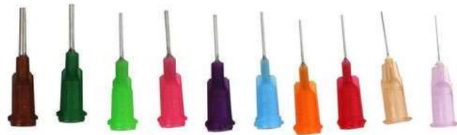
Figure 12. Color syringe needles which can be introduced into samples for Identification and orientation, indicating one side (removed from https://www.esslinger.com ).
