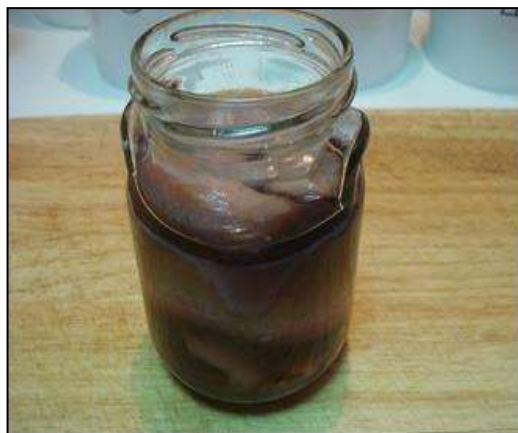
Figure 8. Inappropriate, narrow-mouth bottle.
