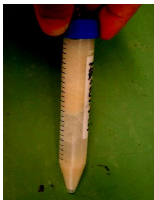
Figure 7. Segregation of a salt hydrate 19]
