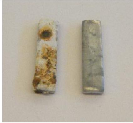
Figure 9. Galvanized steel treated with an eutectic salt water mixture. From left: After treatment and before treatment[20]
