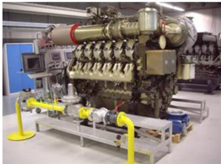
Figura 4. Motor MTU a gas
