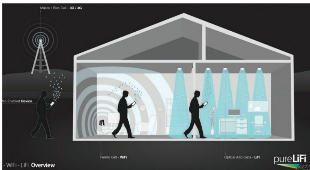
Obr. 2.12: Princip Li-Fi - Atto buňky [38].
