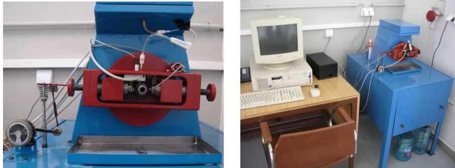
Fig. 1 Device for monitoring of tribological characteristics.
