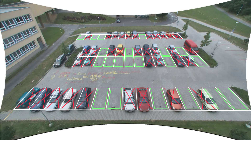
Figure 7.2: Parking lot with highlighted states of parking places as obtained from our method with both contextual constraints and background color model
