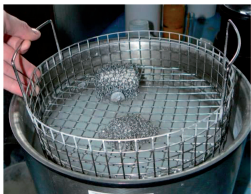
Fig. 6. Cleaning of metallic filters in ultrasonic bath
