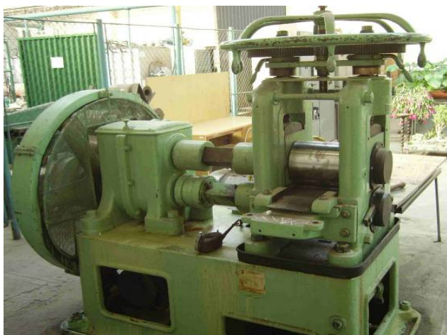
Fig.2. Two-high rolling stand DUO 210 SVa.
