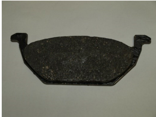
Figure 9: Prepared G6C brake pad.
