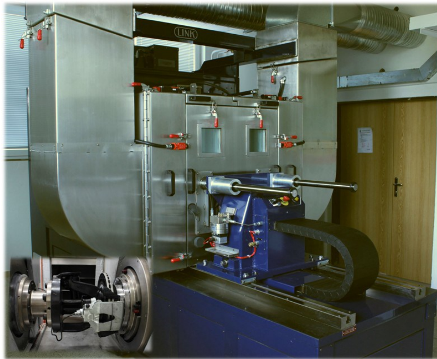
Figure 10: Dynamometer Link M2800 (VŠB – Technical University of Ostrava) with detail of inside part.
