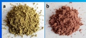
Fig. 1: Composite containing silica frustules and biosynthesized Au nanoparticles (a) before and (b) after calcination
