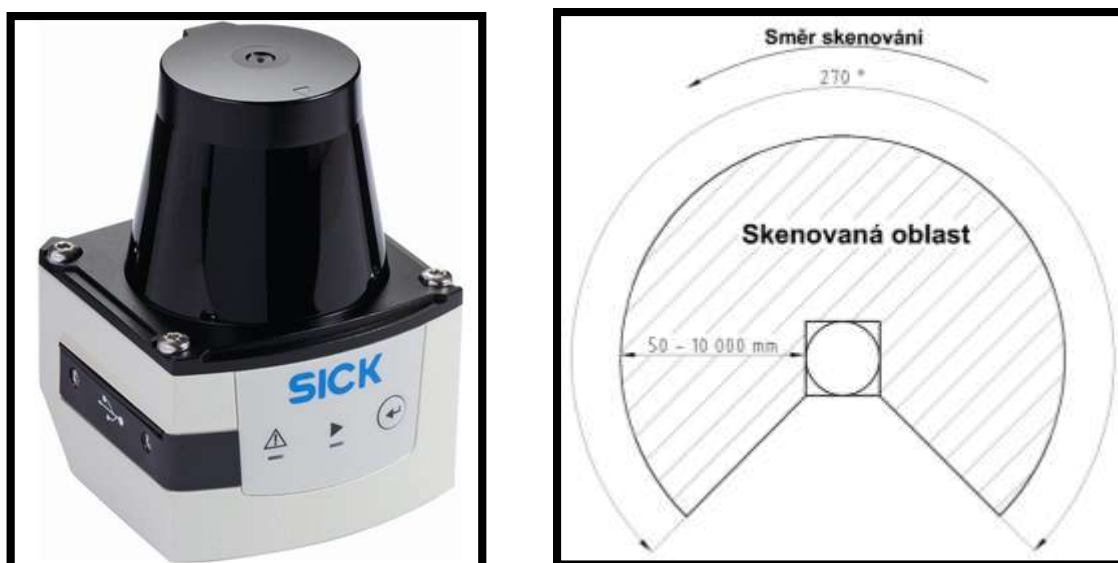
Obr. 3.6 - Laser SICK TiM310-1030000 a skenovaná oblast
