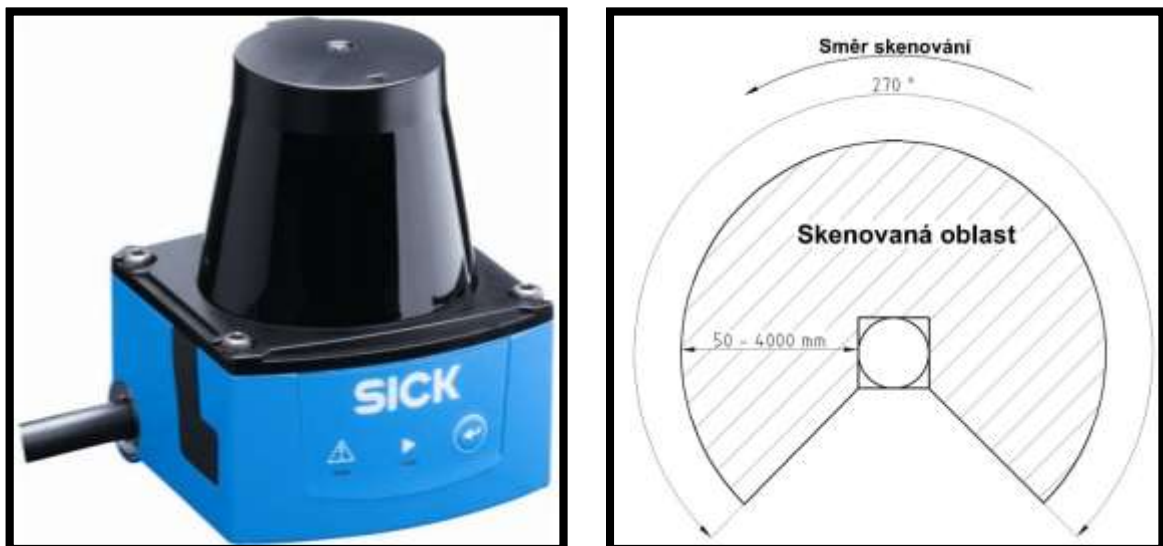
Obr. 3.4 - Laser SICK TiM310-1030000 a skenovaná oblast
