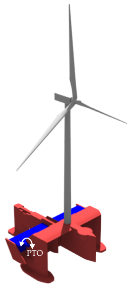
Figure 1. Illustration of the Floating Power Plant P60 device. The red color indicates the foundation, and the blue color indicates the floaters (power take off (PTO)).
