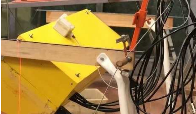
Fig. 3. Experimental method to calculate centre of gravity
