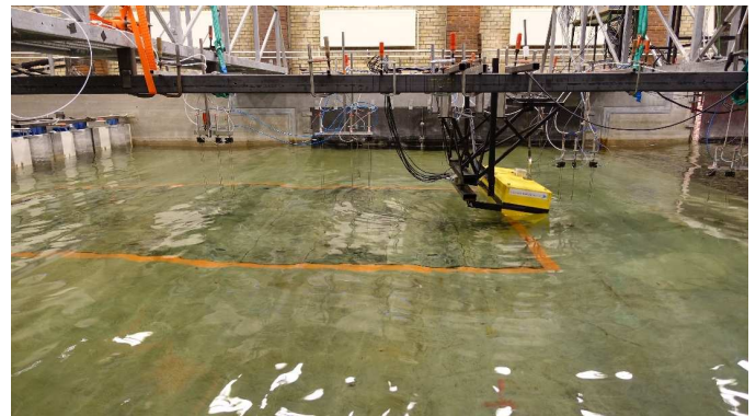
Fig. 8. Experimental setup of single WEC in wave basin
