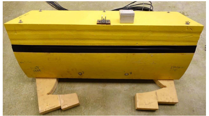
Fig. 2. Stern of WEC showing two of the pressure sensors
