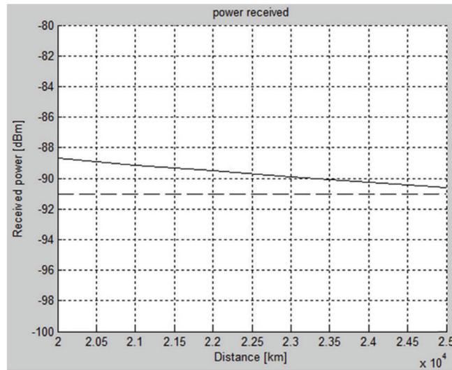
**Figure 3** Received power at the antenna of the eNodeB located at the balloon from a typical LTE mobile phone (the solid curve) according to Friis formula (1). The dashed line indicates the -91 dBm level.
