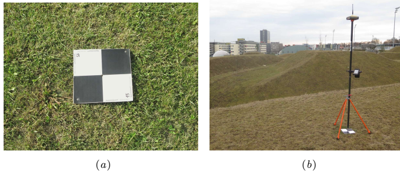
Figure 6. A detail of a ground target captured from the ground (a) and the process of the position measurement using survey-grade GNSS receiver (b). Location: 49°13'44.48"N, 16°34'16.14"E — WGS84.
