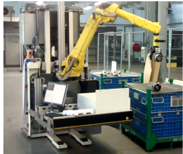
Figure 1: A robot operating in a factory environment using the integrated system. The robot is executing a six-step plan to place two parts in the white kitting box it is carrying.
