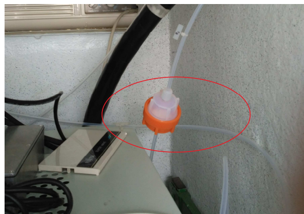
FIGURE 2. Placement of PTFE filter in continuous analyser of tropospheric ozone.
