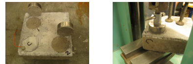
Figure 3 Photographs Showing Pull-off Bond Tests
