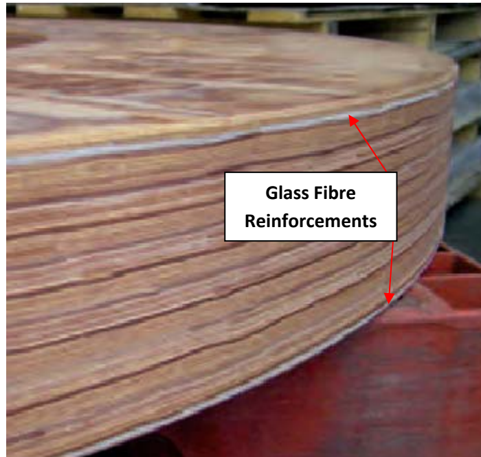
FIGURE-6.41: Laminated Wood Reinforced with Glass Fibre
