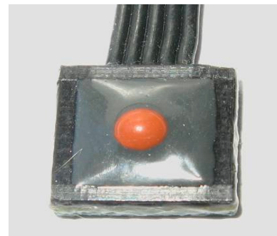
Figure 1 Previous design: SEM micrograph of the bare sensor (on the left) and the mounted and covered chip (on the right).
