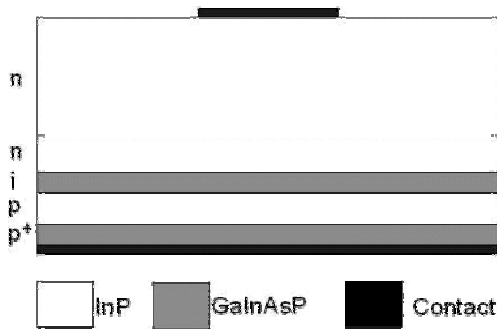
Figure 1 Schematic cross-section of an InGaAsP/InP double heterostructure diode.
