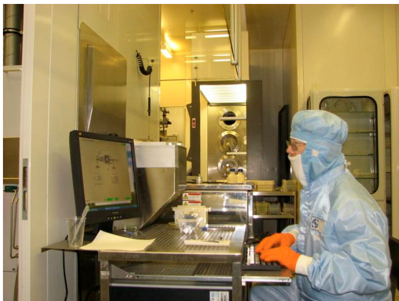
The load-lock and computer control of Oxford Plasmalab 100 DRIE system
