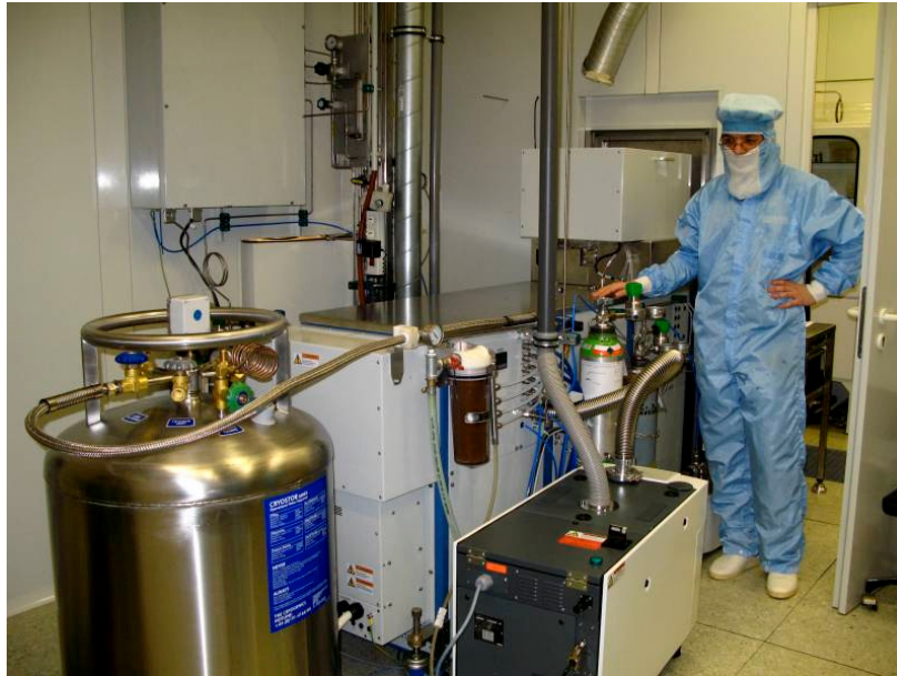
The recently installed Oxford Plasmalab 100 DRIE system
