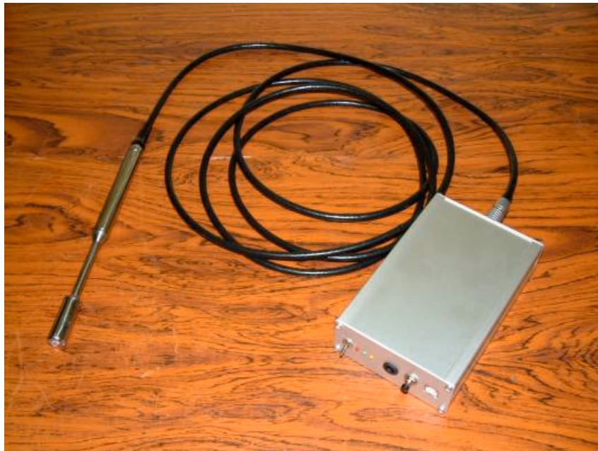
Figure 2 The magnetic probe and the digital signal processing unit.
