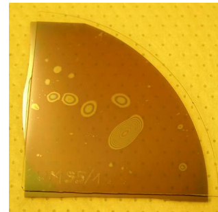
Figure 3 Glass to glass anodic bond with deposited Si intermediate layer
