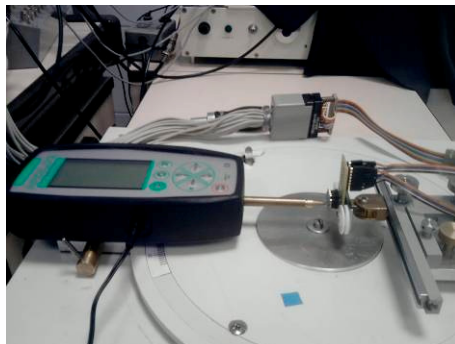
Figure 6 The measurement set-up with the force gauge and the chip
