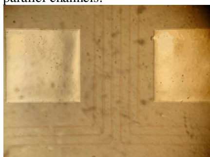
Figure 3 Fluid flow in the 6 parallel channels over the sensing area of the optical structure.
