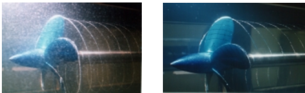
Figure 2: Typical cavitation pattern in seawater (Left) and in freshwater (Right) for water with 40% air content during the cavitation inception test.
