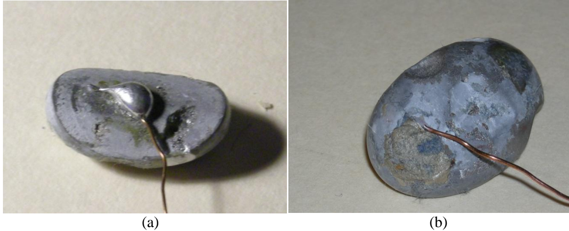
Figure 3-9: (a)-The metallic side of the robin's egg sample showing a soldered copper wire. (b)-The side with the crusty of embedded crystals showing the first of two conductive epoxy layers next to the tip of a copper wire whose diameter is approximately 0.5 mm; the copper wire's tip was sandwiched between the first epoxy layer and a second epoxy layer.
