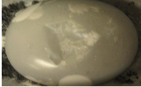
Figure 3-7: The robin's egg sample with an h-BN crust on the metal surface exposed to ammonia during heating. The bottom side which was in contact with the crucible, was bare metal without any h-BN crust.
