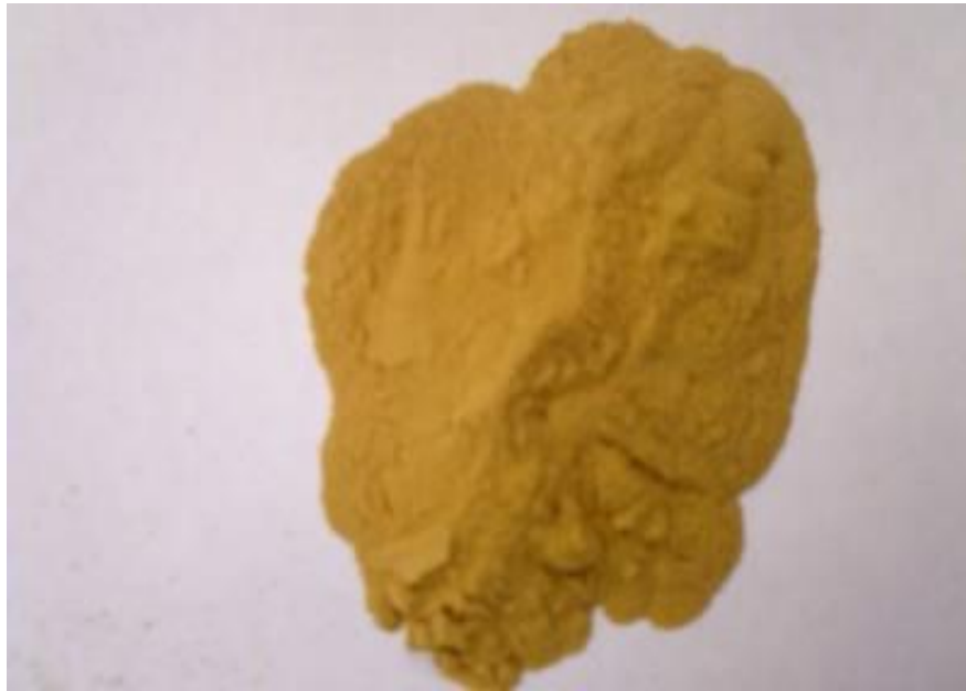
Figure 2-2: Calcium lignosulfonate in brown powder form.
