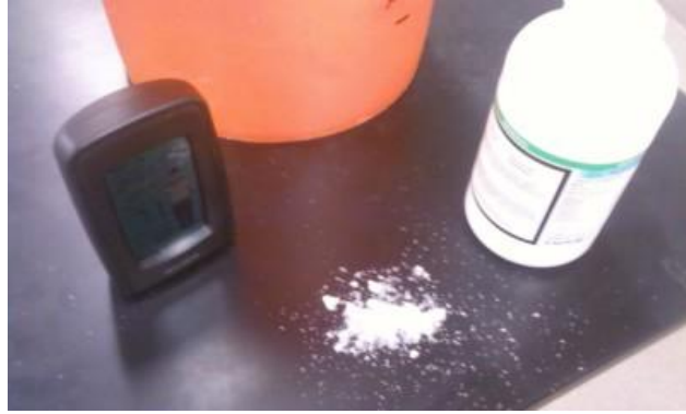
Figure 3-27 Five gallon bucket, magnesium chloride salt, and humidity gauge.
