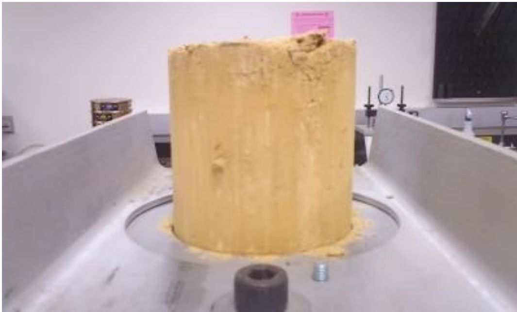
Figure 2-7: Lignin proctor subspecimen at 5% moisture content.
