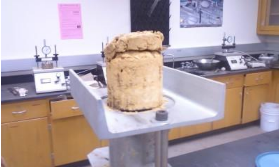
Figure 2-8: Lignin proctor specimen at 15% moisture content.
