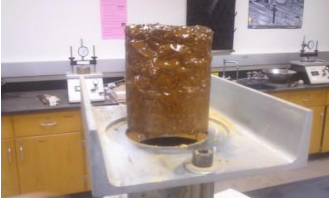
Figure 2-10: Lignin proctor subspecimen at 25% moisture content.
