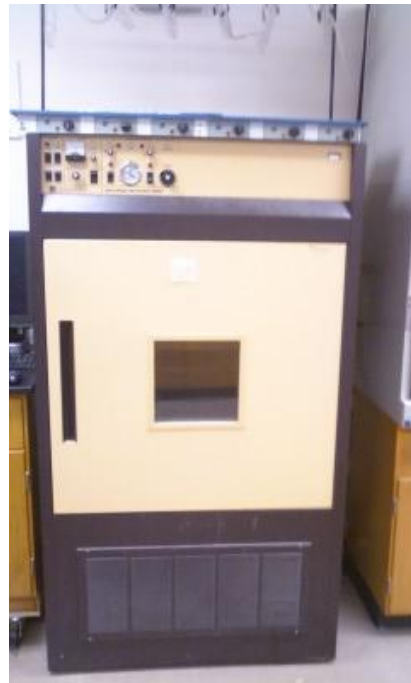
Figure 3-26: Drying incubator for soil samples.
