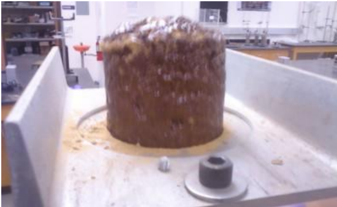
Figure 2-9: Lignin proctor specimen at 20% moisture content.
