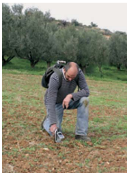
FIGURE 2. Analysis in progress using the hand held portable XRF. The supply cylinder for the helium purge is transported in the back pack.
