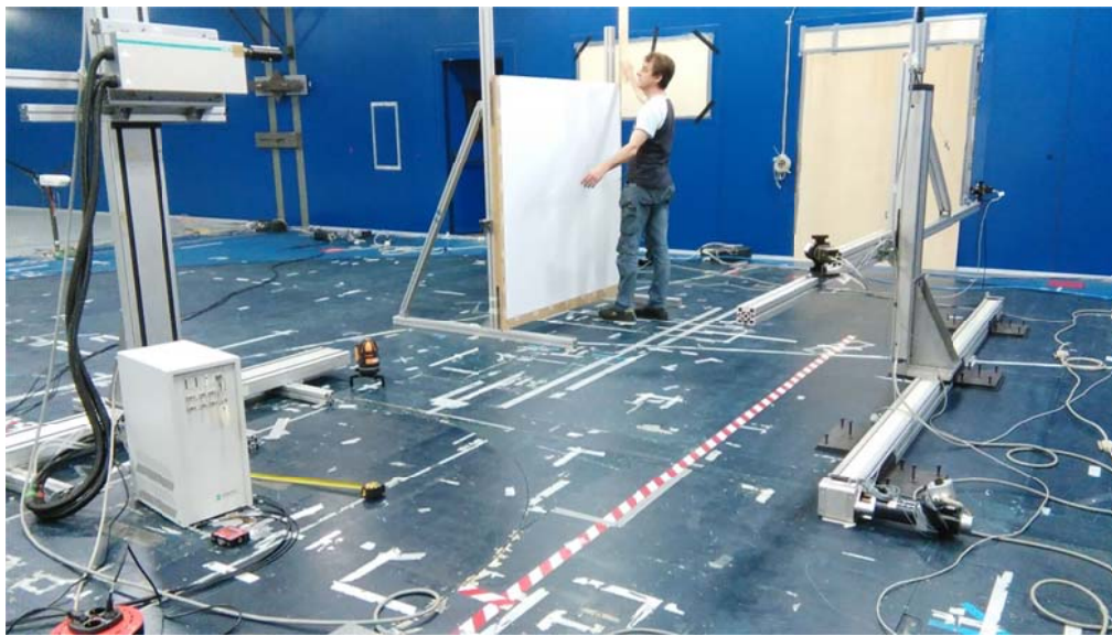
Figure 5: Calibration of the stereo PIV system
