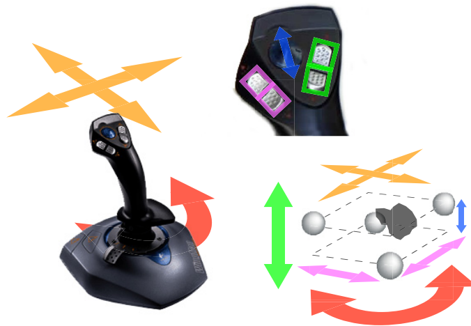
Figure 2. User interface for controlling optical tweezers. A joystick determines the position of a 3D arrangement of trapped silica beads which can be positioned around a target object. Toggle buttons on the joystick control the bead separation which is used to grip the target object. Twisting the joystick allows the target object to be rotated.
