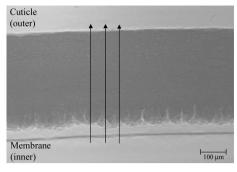
**Figure 2** A typical X-ray transmission image of an eggshell, obtained using the defocused beam. The arrows shows the areas where X-ray scattering patterns were recorded: three vertical scans were made 48  $\mu m$  apart. The vertical scan length was 500  $\mu m$ . Samples were bathed in the direct beam. Differential absorbance allows microscopic features to be observed.
