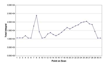
Figure 5 Total integral of scattering intensity at each of the points on the vertical scan. The largest value at point 8 corresponds to the centre of the mammillary layer. An increase in the total integral is seen as the scan progresses towards the outer surface of the shell. The sample thickness was 300  $\mu m$  throughout.
