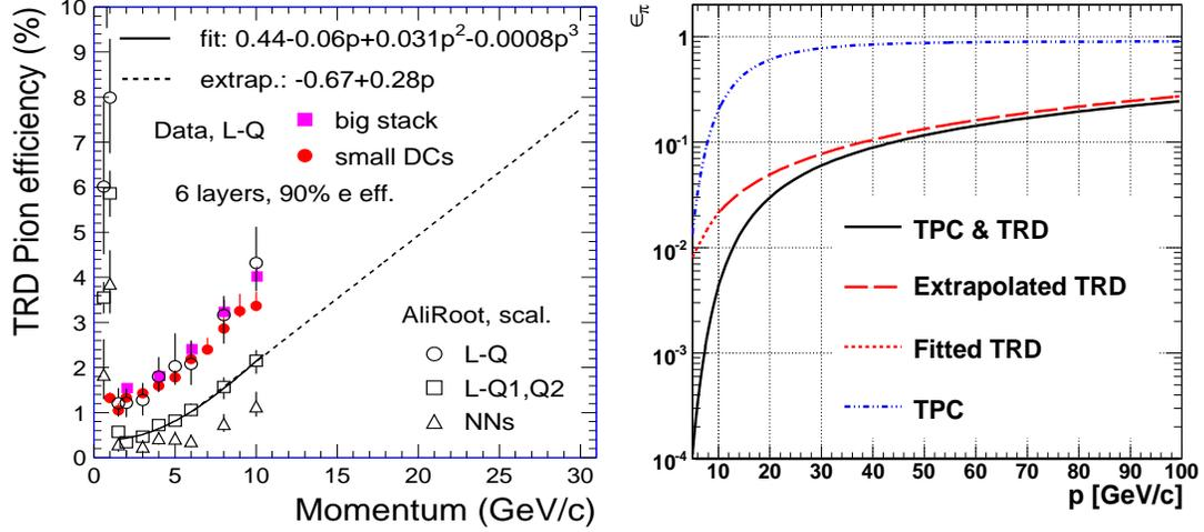
FIG. 1:  $\epsilon_e^{\text{TRD}}$  as function of momentum extracted from testbeam data compared with simulations within the ALICE framework and extrapolated to high  $p$  (left panel). Calculated  $\epsilon_e^{\text{TPC}}$ , extrapolated  $\epsilon_e^{\text{TRD}}$  and combined  $\epsilon_e^{\text{TPC+TRD}}$  as function of momentum (right panel).
