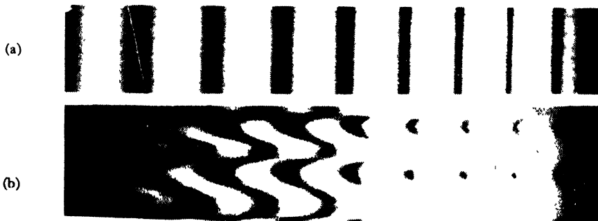
Figure 5(a). Banded spectrum obtained with a crystal of \text{BaSO}_4 ( t = 0.16 cm) kept between crossed polars. The left end corresponds to the red region of the spectrum.
