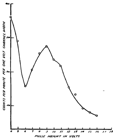
Fig. 6. Differential pulse height spectrum of pulses from stilbene in xylene liquid scintillator due to \text{Co}^{60} gamma rays.
