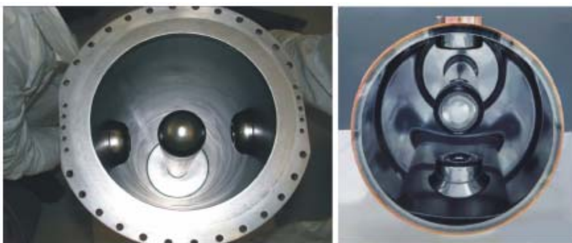
Fig. 11.5: Photographs of the cavities made with the two technologies. The bulk niobium [3] at left and the sputtered niobium at right [4].
