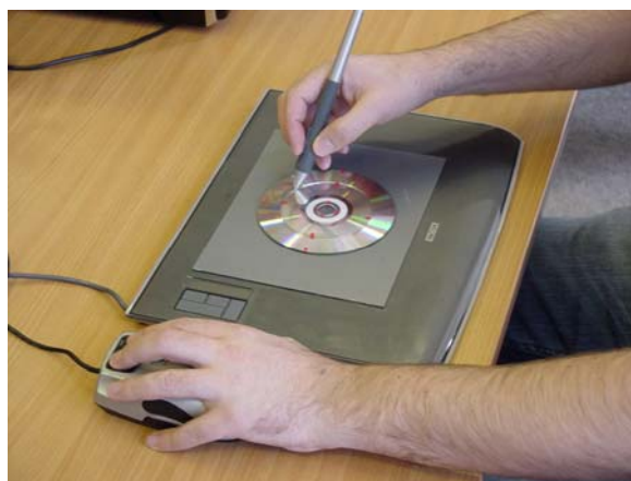
Figure 1: Prototype Tac-tiles system. Graphics tablet augmented with a tangible pie chart relief, with dynamic tactile display for non-dominant hand.
