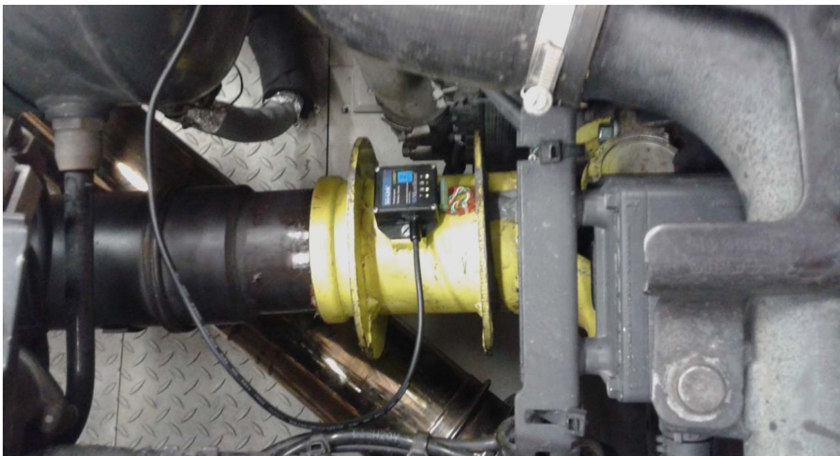
Figure 10: Torque measurement device on the cardan shaft of vehicle #1
