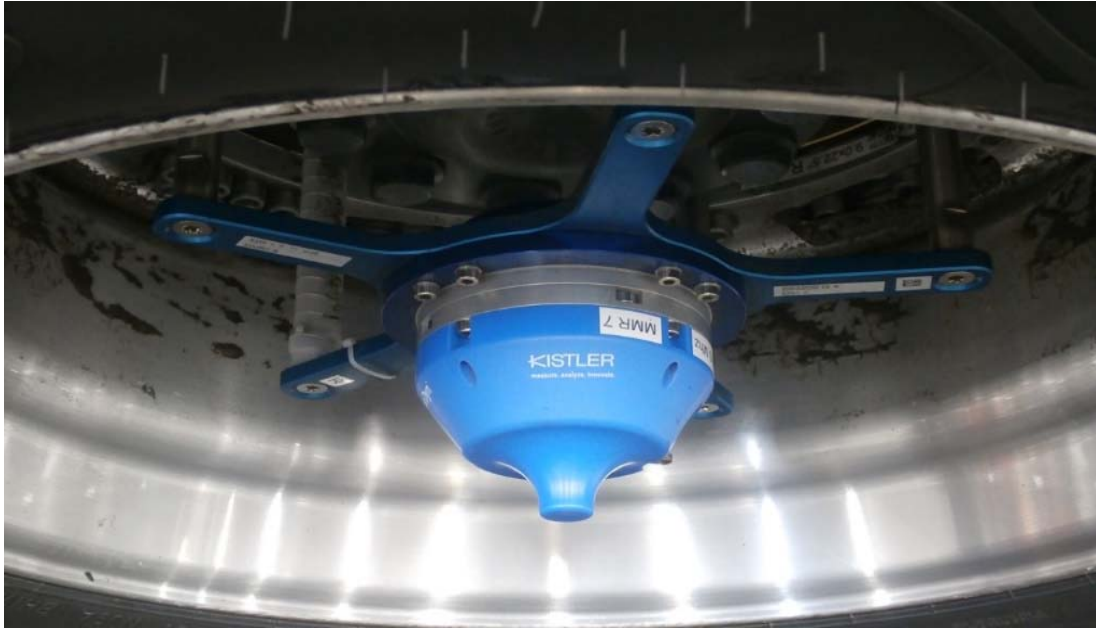
Figure 13: Torque measurement device at the wheels of vehicle #2
