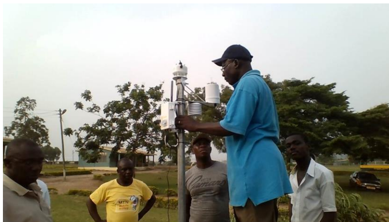
Figure 1: Staff of the Ghana Meteorological Agency installing a TAHMO Generation 2 Weather station at a school in Ghana (Source: Annor et al., 2016)
