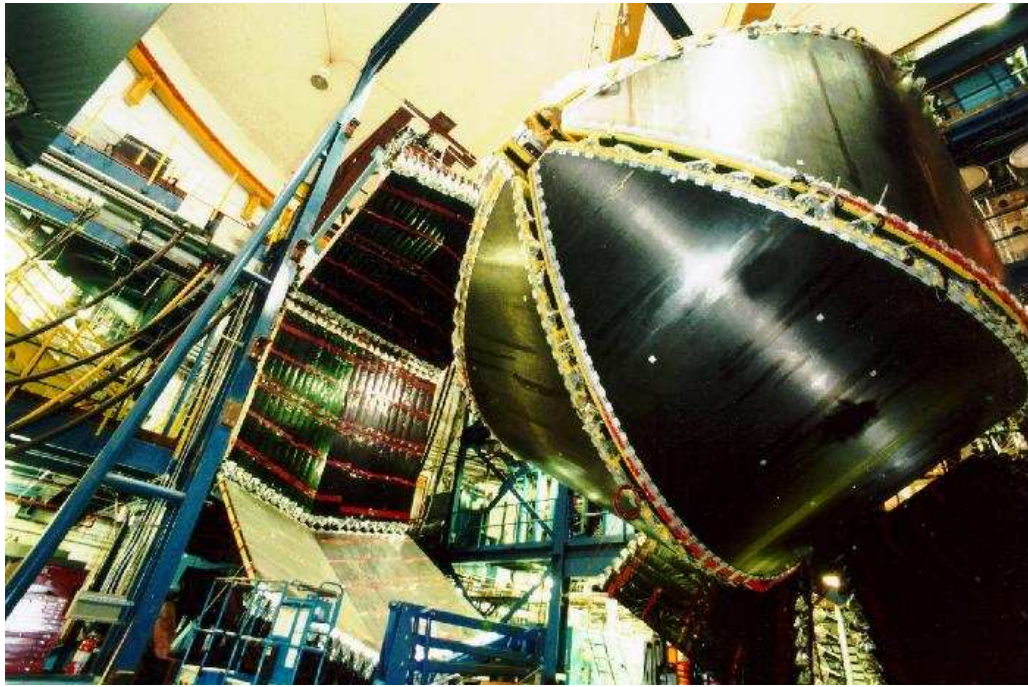
Figure 3.7: The CLAS detector with open clamshell . The six sector configuration of the drift chambers (region 3 visible) can be seen, along with time of flight scintillator paddles (left of centre).
