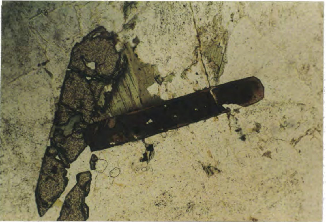
Photo 3.11. Euhedral, prismatic, dark brown-coloured allanite in the quartz monzonite (sample N135) showing zoning. In the field view, there are also titanite, apatite and biotite minerals. The latter is chloritised. Magnification: 1.3x0.77 mm, PPL.
