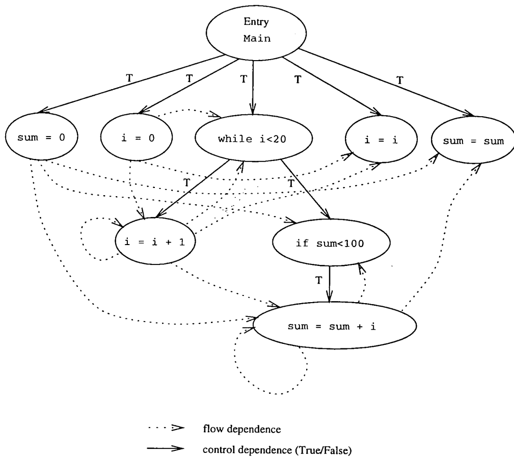
Figure 3.4: Example Procedure Dependence Graph.
