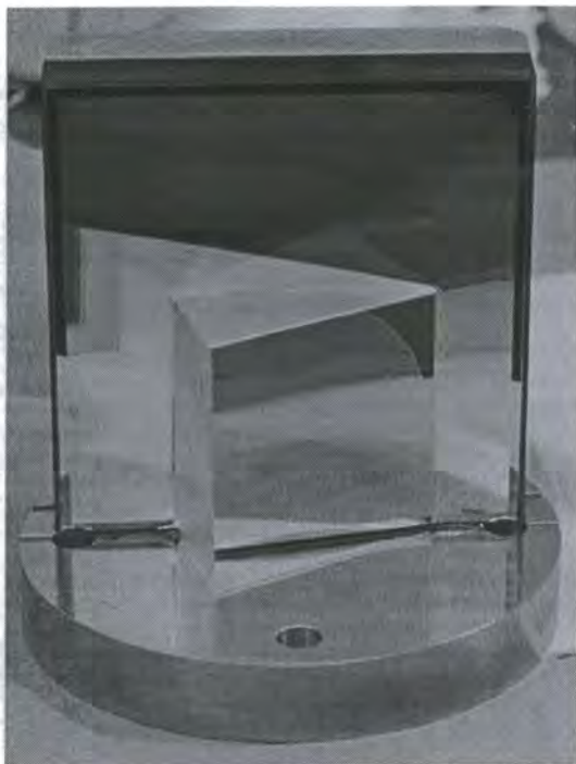
Figure 2.10: Photograph of the immersed grating taken during manufacture. Note the glycerol layer, seen at the top right corner of the prism, has yet to fully expand to the full area of the prism. The immersed grating is seen positioned on the grating mount.
