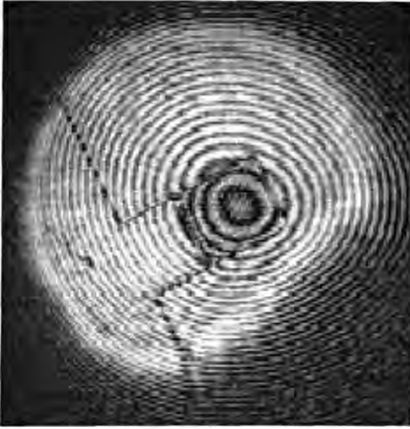
Figure 7.7: Interferogram of SMIRFS-IFU input fibre bundle after polishing. The fringes are centred on the tube array which can be seen as a rectangle in the centre of the interferogram.
