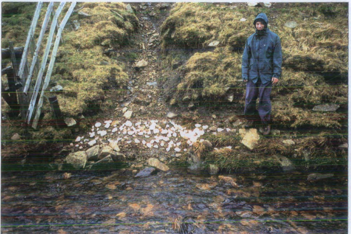
Figure 7.2 Site 2 - Painted tracer pebbles placed at base of cut bank
