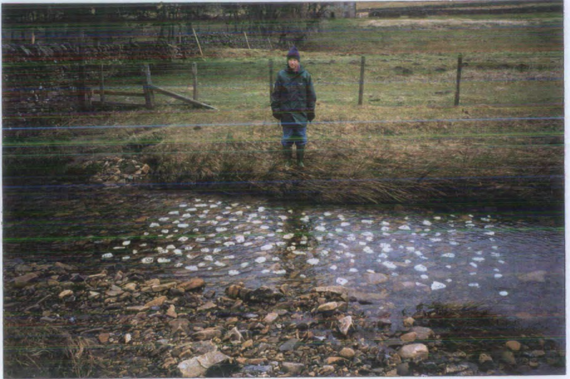
Figure 7.1 Site 1 - magnetic tracer pebbles placed on the channel bed, extending up to four metres upstream of section 1
