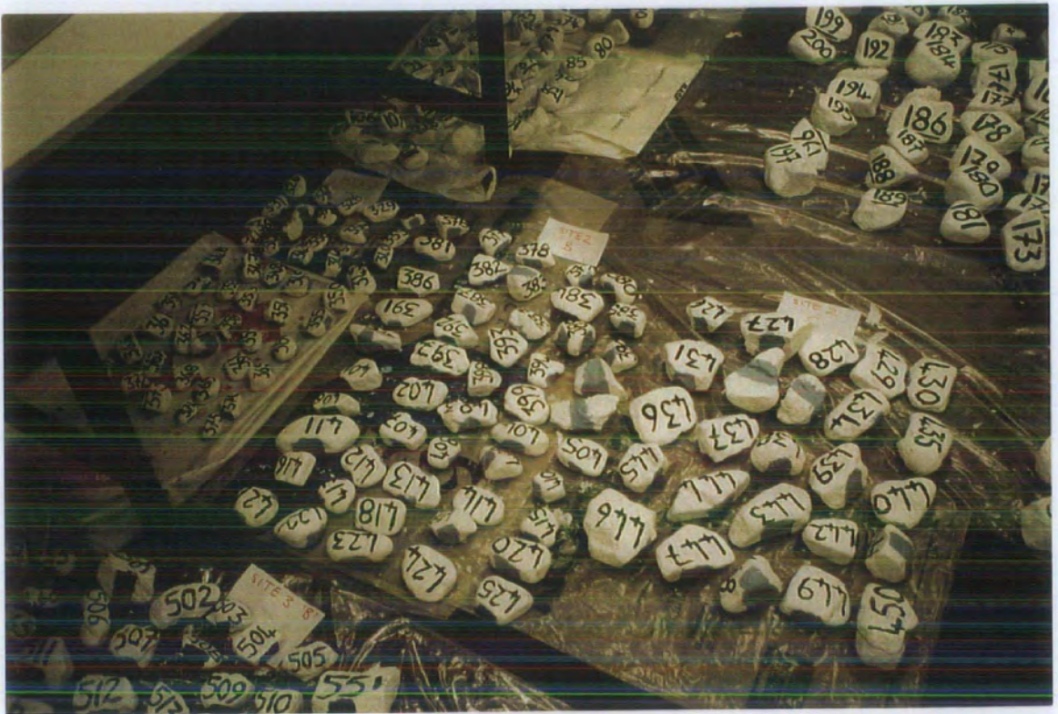
Figure 3.12 Tracer pebbles sequentially labelled with a number in black
