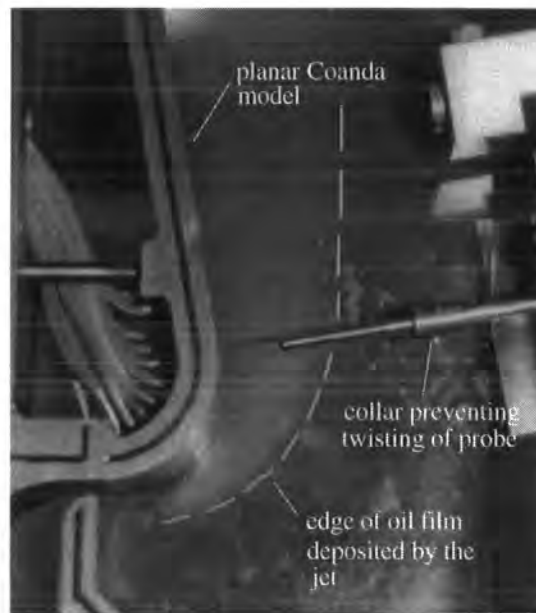
Figure 4.25 : Photograph of the planar model, demonstrating the oil contamination
