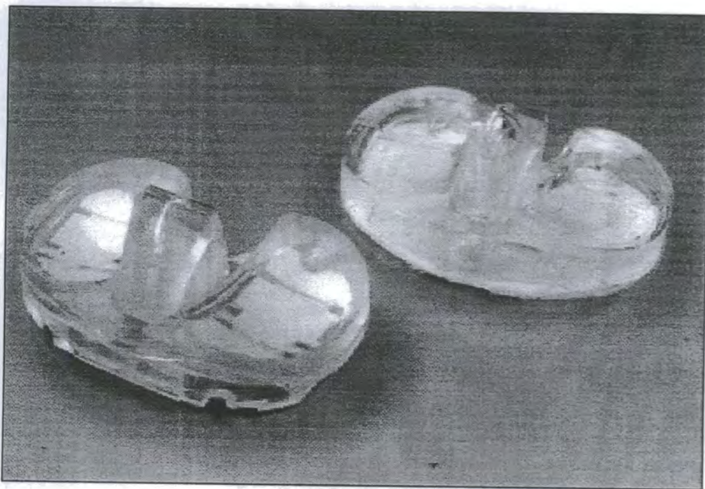
Figure 3.5 Pre-prototype acrylic / PU tibial compliant bearings.
